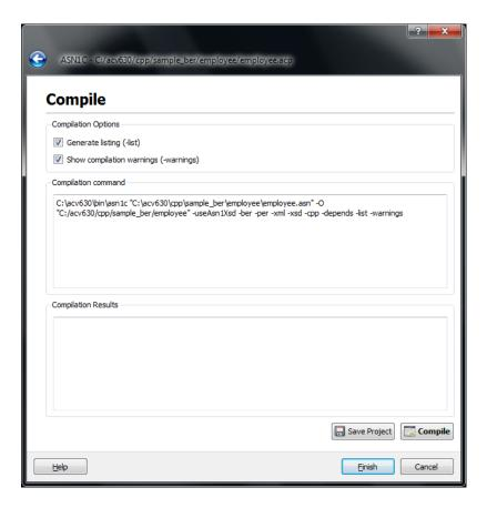
Included in the window are the compiler command, an option to save the project, and the output from compilation. Selected options are reflected in the command line.
